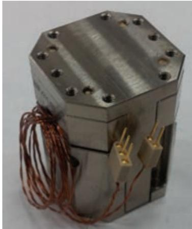
Figure 3.8: A photograph of piezo positioner.
