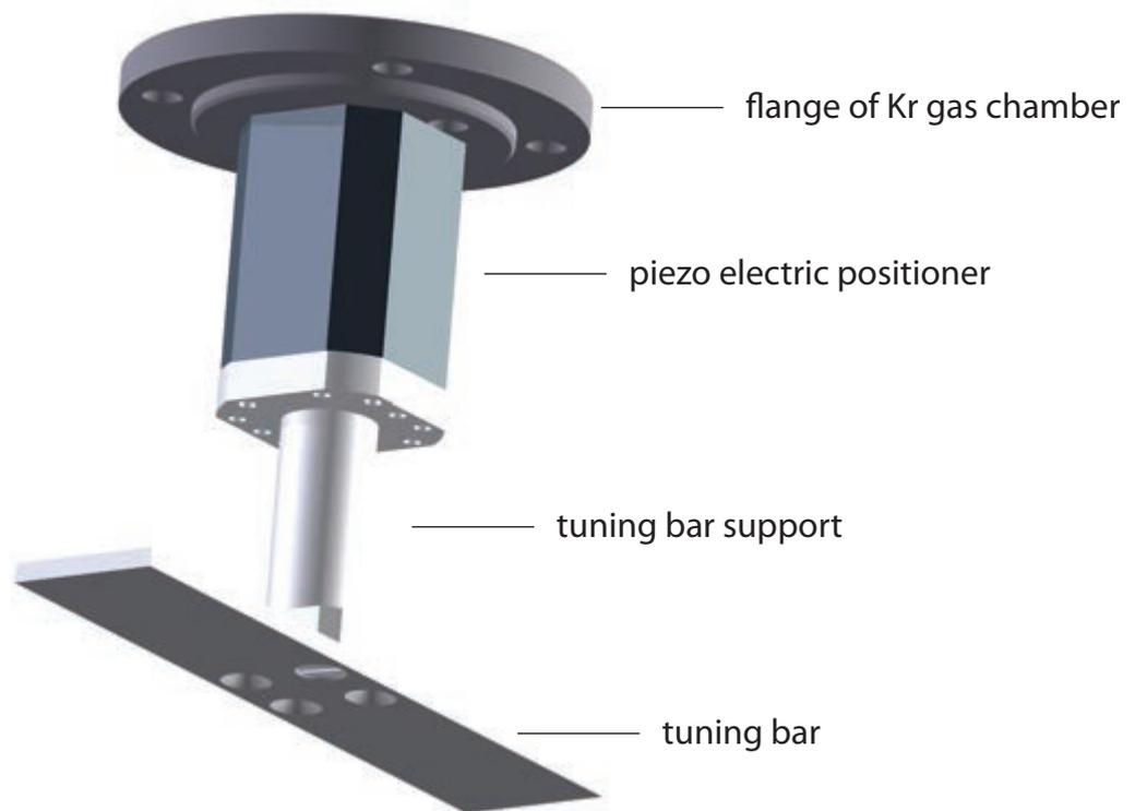
Figure 3.6: A schematic drawing of the tuning bar.
