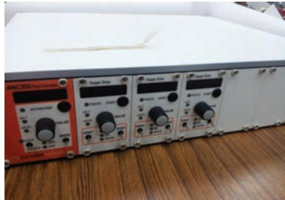
Figure 3.9: A photograph of piezo controller.
