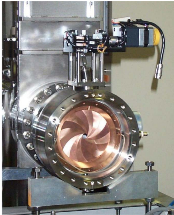
Figure 2.20: Picture of the variable and floatable aperture.
