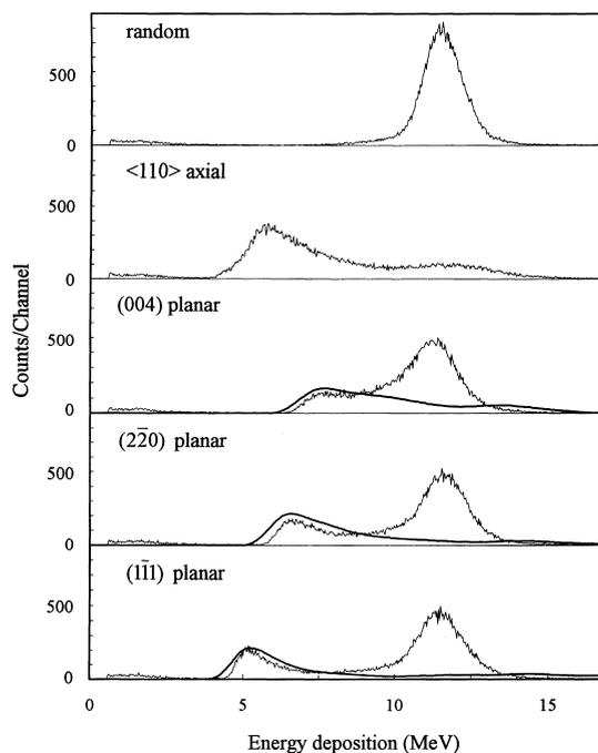
Fig. 1. Spectra of deposited energy to the SSD for random,  $\langle 110 \rangle$  axial, (004), (220) and  $\langle 111 \rangle$  planar channeling conditions. Thin lines are experimental results, and thick lines are simulations.
