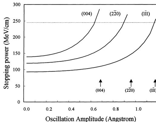
Fig. 3. Relations between stopping power and oscillation amplitude for (0 0 4), (2  $\bar{2}$  0) and (1  $\bar{1}$  1) planar channeling 290 MeV/u  $C^{6+}$  ions. Dotted line indicates random stopping power, and arrows indicate positions of channel walls.
