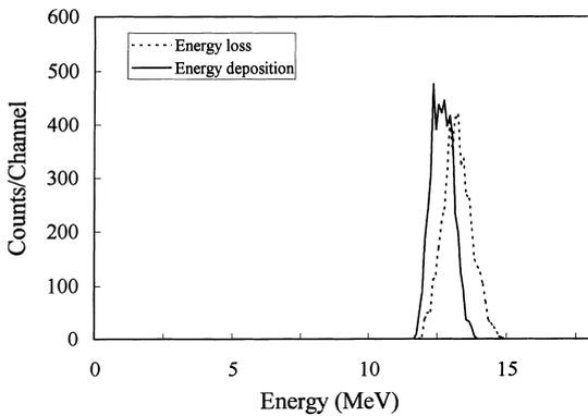
Fig. 2. Spectra of simulated energy loss (dotted line) and energy deposition (solid line) for the random direction.
