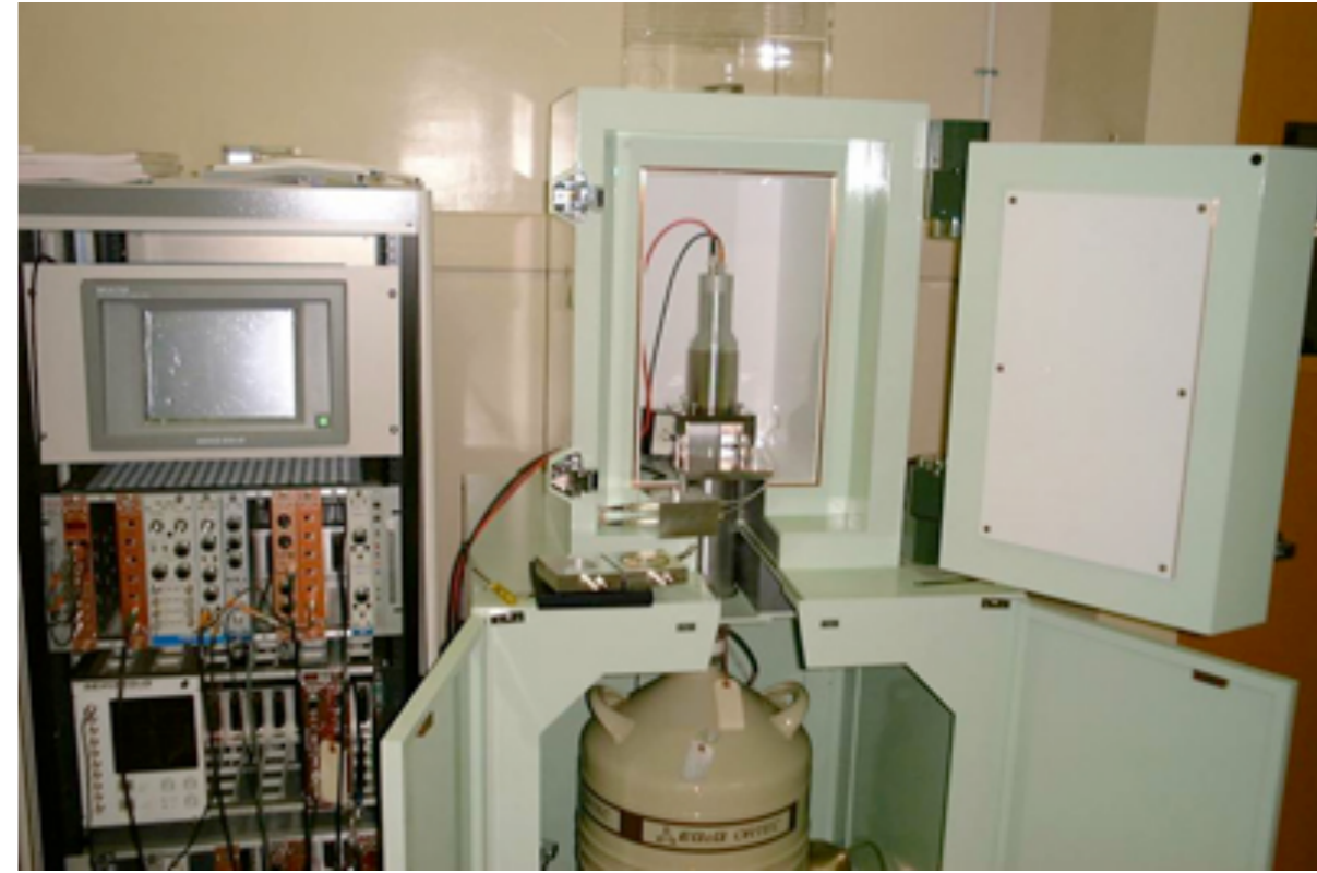
Ge detector for check of food samples
