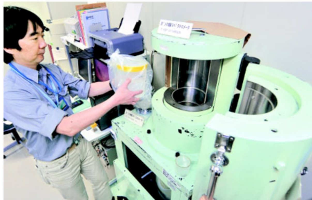
Ge detector for check of food samples
