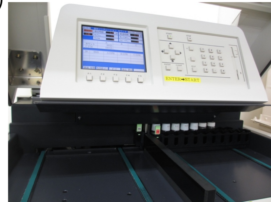
liquid scintillation counter
